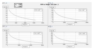
Fig. 5. Results: Test Case - 2, ((SNR vs Range at ID = 100 and n = 100)
